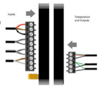
Once all sensors have been attached, simply press the removable connector into the base unit.
